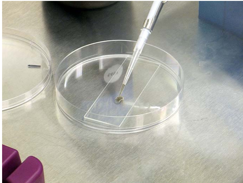
Image 2: Inoculation of carrier with 0.020 ml of Aspergillus brasiliensis.
